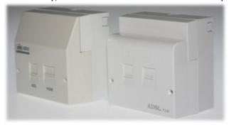
If you have a faceplate which sticks out, then it's likely to be an ADSL filter faceplate. These allow you to filter all your telephone extensions in the master socket, which means you don't need individual microfilters on each phone extension socket. If you have one of these then remove it to reveal your test socket (Be careful when doing so as your internal wiring if you have any, will be attached to the rear of this plate)...
